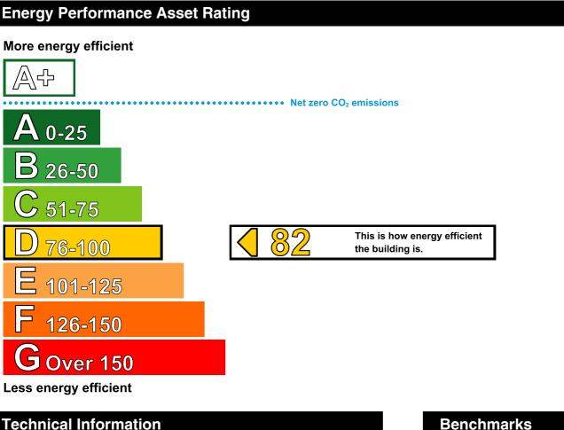
Oil Main heating fuel: Building environment: Heating and Natural Ventilation 1031 Total useful floor area (m<sup>2</sup>): Building complexity (NOS level): 3 Building emission rate (kgCO<sub>2</sub>/m<sup>2</sup>): 40.55
